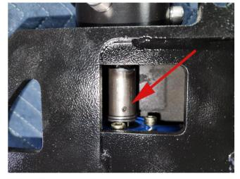
Verify the driveshaft is scure to the gearbox with a 5/64 Allen wrench
