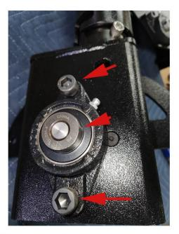
Remove the bearing from the housing opposite the fender side, using a 3/8" Allen wrench. Loosen the 2 set screws, securing the axle with a 1/8" Allen wrench
