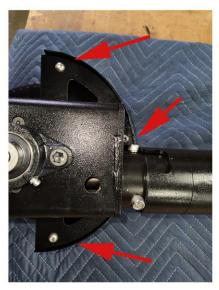
Remove the 3 cap screws securing the fender, using a 3/16 Allen wrench.
