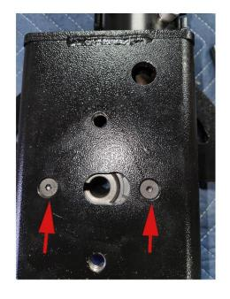
Remove the axle and remove the 4 flathead screws, on both sides of the housing, securing the gearbox, using a 5/32 Allen wrench
