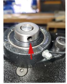
Loosen the two set screws on the bearing mounted on the fender, using a 1/8" Allen wrench
